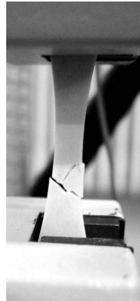
Fig. 5. Failure of a facies sample after dynamic testing (1 m/s).
